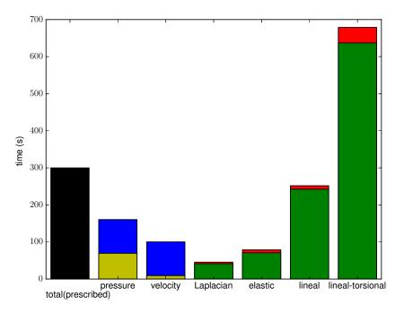
Figure 6: Breakdown of profiling data for the Fluidity implementation of the mesh movement methods for the oscillating cylinder problem on 24 cores of the ARCHER HPC system. The black bar shows the total runtime for the fluid solver, using prescribed mesh movement, with further splits for the pressure and velocity solves, coloured by matrix assembly (blue) and linear solve time (yellow). This is compared against the assembly (red) and solve time for four mesh movement algorithms.
