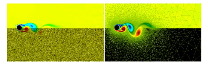
Figure 3: Two snapshots of the oscillating cylinder problem for different mesh movement methods. The left image shows the result with prescribed mesh movement, without hr-adaptivity, the right uses viscous drag mesh movement with an hr-adaptive mesh. The number of degrees of freedom in each is approximately equal. Here a case for a oscillation amplitude of 0.15 cylinder diameters (a small displacement case) and f = 0.22 is shown.
