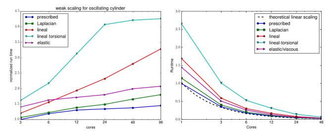
Figure 5: Weak (left) and strong (right) scaling results for the various r-adaptivity methods performed using Fluidity on the ARCHER HPC system. 'Prescribed' refers to the analytical method of defining the mesh velocity as described in section 5.2, while the other methods are as described in the appendix.
