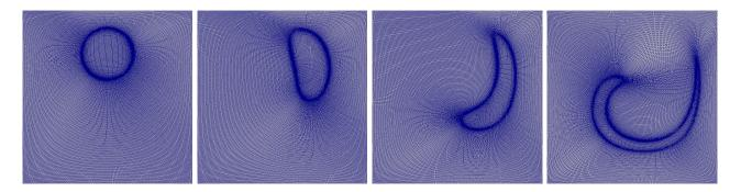
Figure 1: Meshes at a series of time levels computed using r-adaptivity only for the advection problem.
