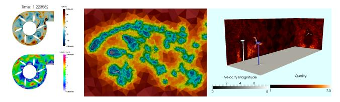
Figure 4: Images showing physical applications of the new functionality in Fluidity, from left to right: vorticity and velocity fields for an idealised 2D centrifugal blower; mesh size from an hr-adaptivity simulation of a 2D slice through a rotating Darrieus style vertical axis turbine; and a 3D simulation of mesh quality and flow past a horizontal axis wind turbine.
