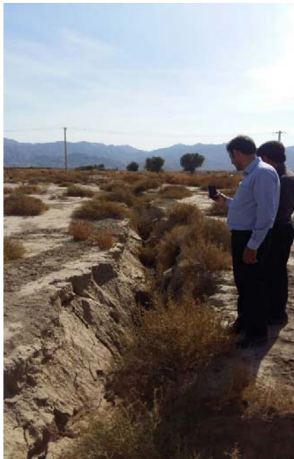
Fig. 6 Creating a gap and seam due to undue and uncontrolled use of groundwater
