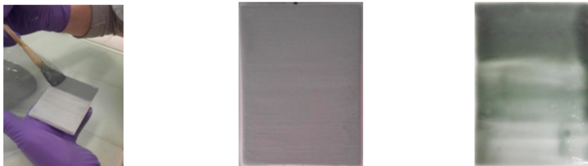
Figure S3. (a) Example of colored coating deposition. (b) pre-fired condition. (c) Glaze after firing.
