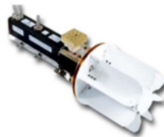
Fig. 1 Traveling Wave Tube Amplifier Device- Ku Band TWT [2] (courtesy of L-3 Comm. Electron Technologies Inc., CA)
