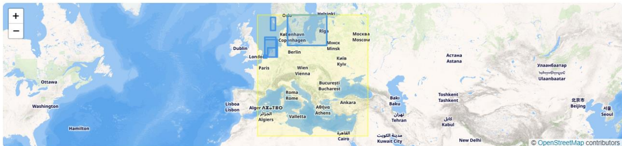
Figure 12 - Map interface using OpenStreetMap. The yellow box indicates the bounding box chosen by the user. The blue boxes are the resulting data sources found.
