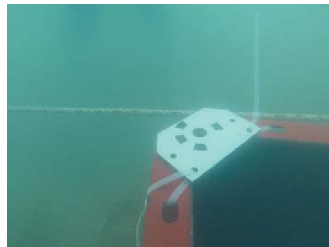
Fig. 10 Image showing the use of Agisoft Potoscan Pro markers for better automatic alignment in processing (Photograph Felix Pedrotti)
