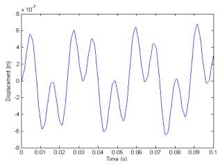
Fig. 2 Analytical solution of forced vibration problem exposed to cosine force
