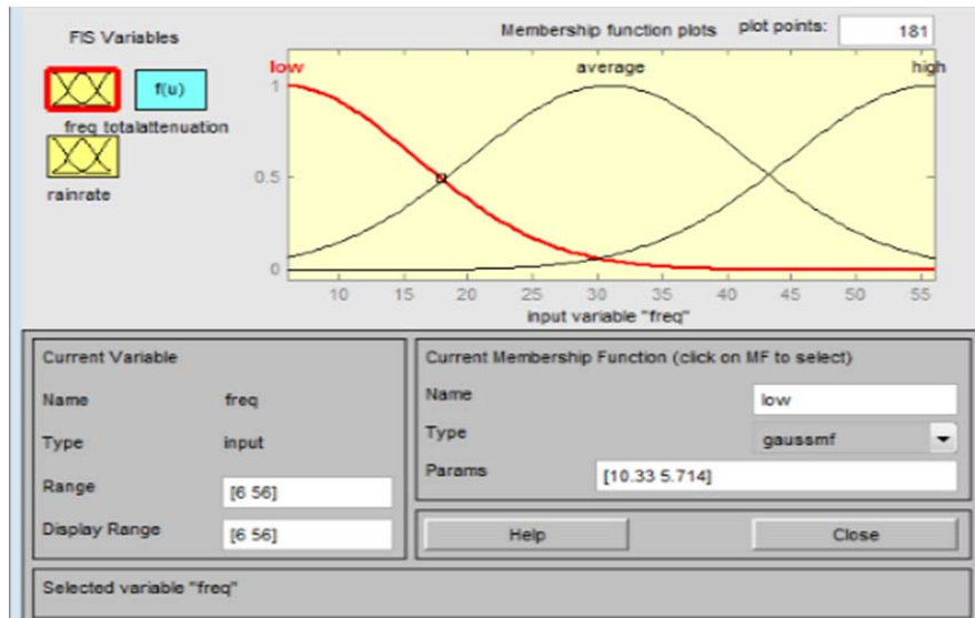
Fig. 3 A typical MF for rain attenuation values at different rain rates and frequencies
