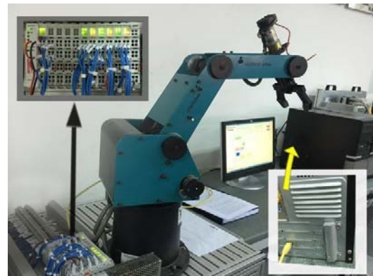
Fig. 7 Control system and robotics arm installation
