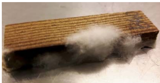
Fig. 5 Wood sample which has just been harvested from the petri dish, where the mycelium has not still been brushed off
