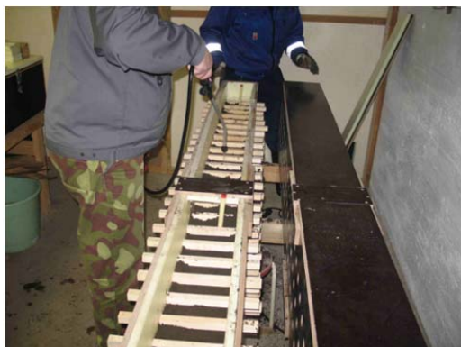
Fig. 6 Setting wood samples to the soil-box used for accelerated soil contact durability testing. The specimen penetrating the box will be entirely covered with moist soil mimicking the ground contact tests for several weeks
