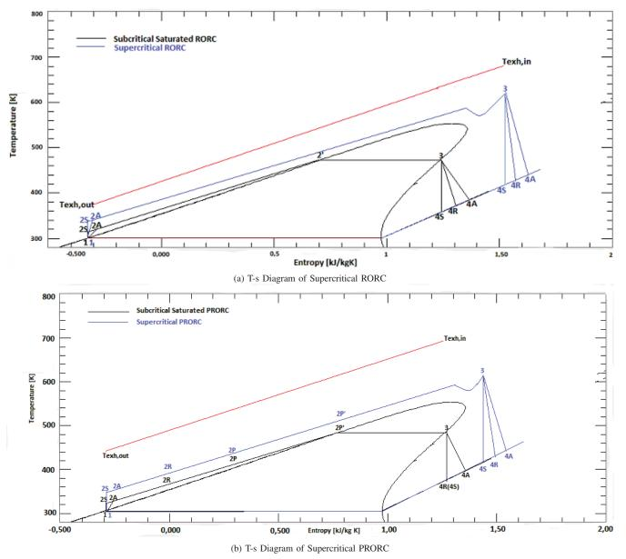
Fig. 2 Supercritical RORC and PRORC Configurations
