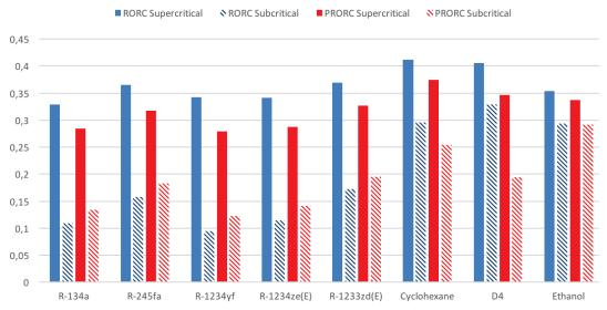
Fig. 3 Thermal efficiency for RORC and PRORC
