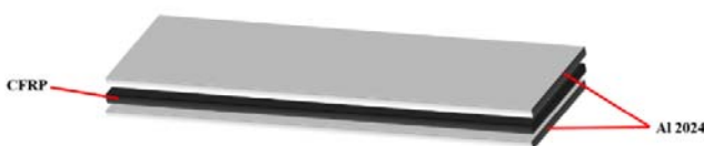
Fig. 2 Layup of each FML for single lap joint
