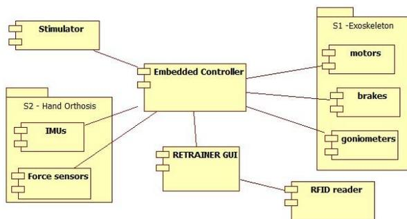
Figure 3. RETRAINER system architecture
