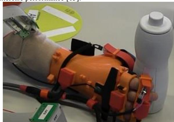
Figure 2. Hand orthosis interacting with a smart object
