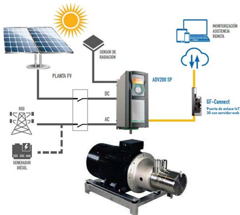
Figure 14. Scheme of the configuration for zero energy discharge using the VFD DC bus.
