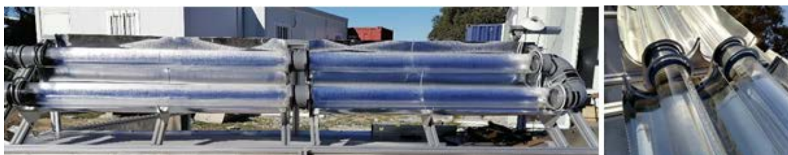
Figure 67. Reactor with the four horizontal receivers.
