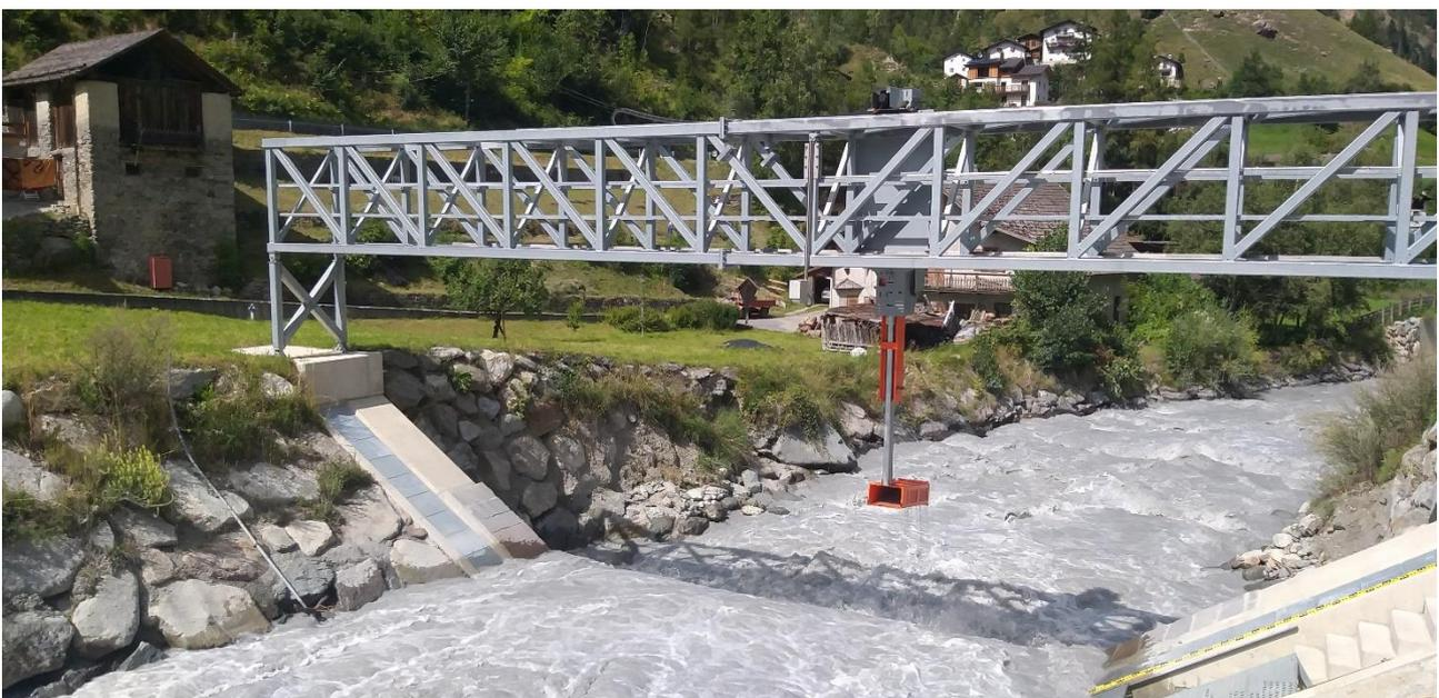
Figure 1. View of the BLS during the lifting of the mobile trap sampler.
