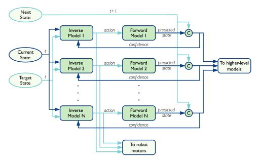
Figure 3: Overview of the HAMMER architecture.
