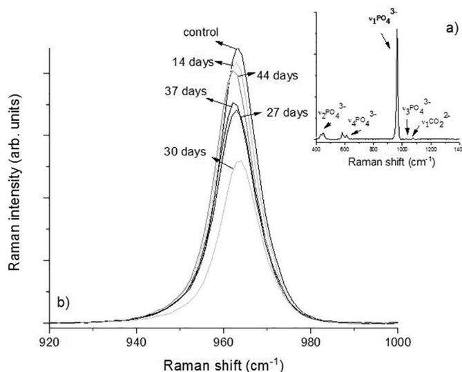
Fig. 2. a) Raman spectrum obtained for control sample B2; b) comparison of the baseline-corrected spectra obtained for sample B2, before treatment and at days 14, 20, 27, 30, 37 and 44.
