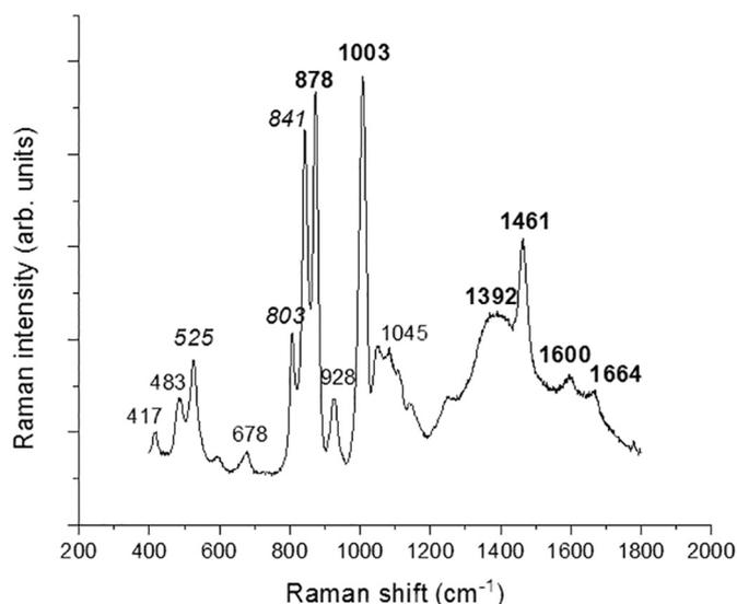
Fig. 1. Raman spectrum obtained for a drop of whitening agent.
