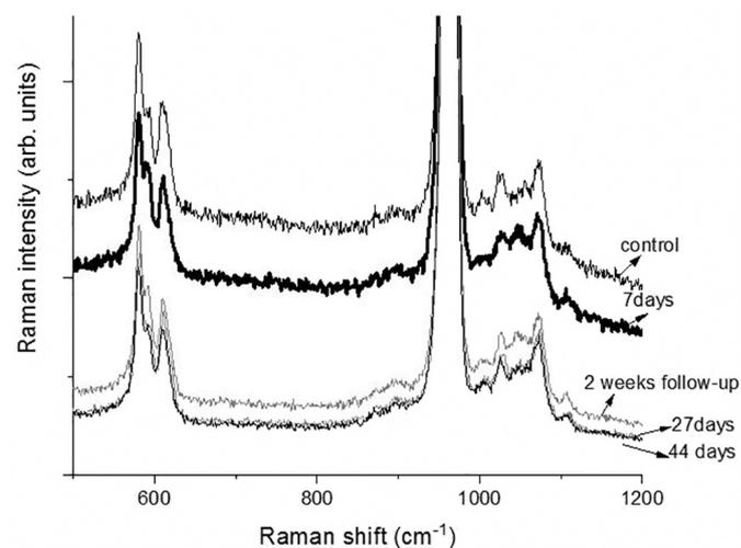
**Fig. 4.** Comparison of the Raman spectra background obtained for sample A3, without baseline correction, before treatment and at days 7, 27, 44 and 2 weeks follow-up.
