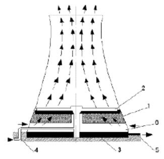
Fig.1. Configuration of natural draught cooling tower with counter-flow. 1-water-catcher; 2-water distribution system; 3-cold water pond; 4-hot water inlet; 5-cold water output; 6-air feeding.
