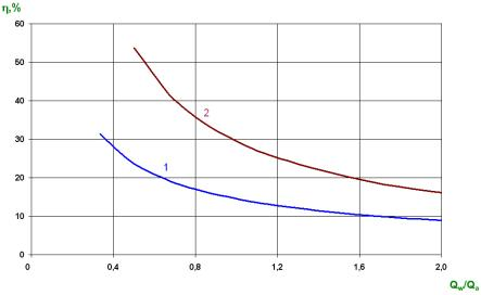
Fig. 3. Thermal efficiency of the use of low-grade heat in cooling towers with an inner (1) and external deployment (2) of the packing depending on the ratio of the intensity of water  $Q_w$  and  $Q_a$  of air flows.
