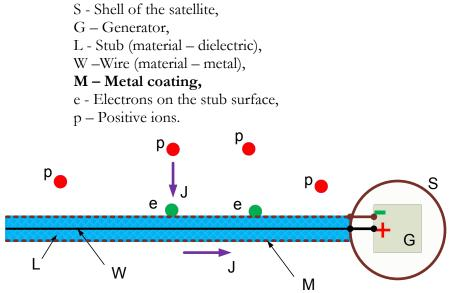
Fig. 1. The stub is connection to the generator.
