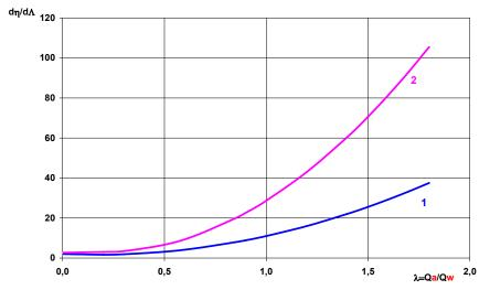
Fig. 4. The rate of increase of thermal efficiency  $d\eta/d\Lambda$  ( $\Lambda = Q_w/Q_a$ ) in the two cooling towers - with an inner (1) and outer (2) heat transfer when the relative flow configuration is changed.
