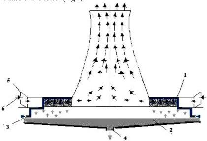
Fig .2. Configuration of natural draught cooling tower with cross - flow. 1 –packing ; 2- pond;3- entrance of warm water ; 4 output chilled water; 5 air adjustment boards; 6 - entrance of outside air.
