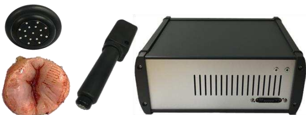
Figure 1: Impedance spectroscopy with multiple electrode probe and excised cervical tissue (normal case).
