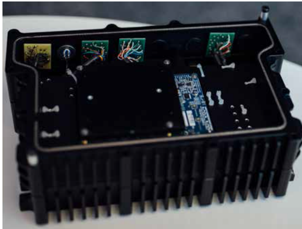
Figure 3: SOTAS Vehicle Tactical Server Platform (VTSP) rev 2 Hardware
