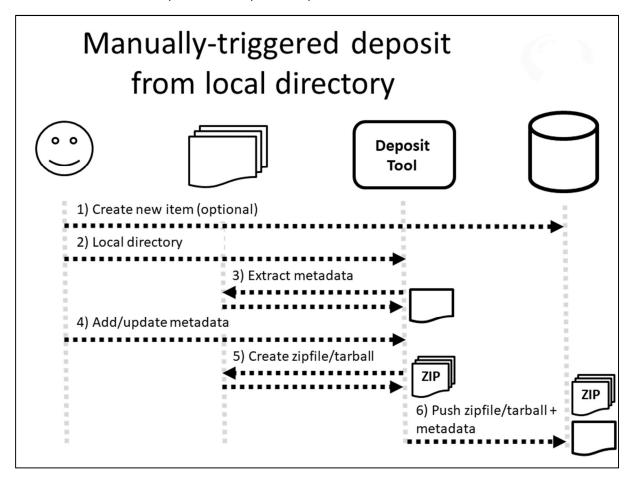
Within this workflow, a researcher requests that a deposit of their software be made. The deposit tool creates a zipfile/tarball of a folder containing the software, compiles associated metadata and makes the deposit into the digital repository.
