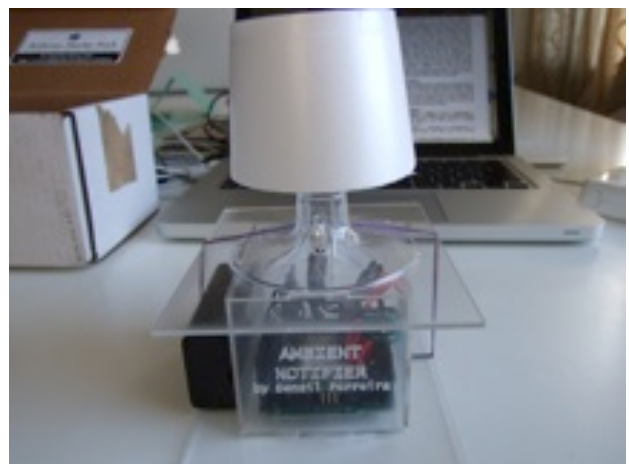
Figure 3. The Arduino board is installed in an acrylic case underneath a lamp. The LED light shines through the case and lights up the lamp overhead.
