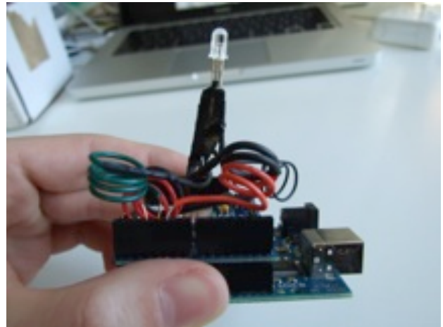
Figure 1. And RGB LED connected to an Arduino Duemilanove via a 220 Ohm resistor forms the basis of the Ambient Notifier.
