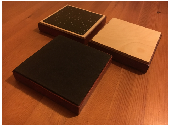
Figure 1: Non-functional prototype instruments. Clockwise from right: #1 (wood), #2 (foam rubber), #3 (capacitive sensor)
