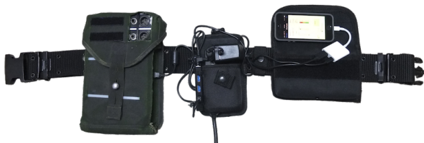
Figure 9: robotcowboy belt hardware 2017 left: USB audio interface, center: USB hub, right: iPhone
