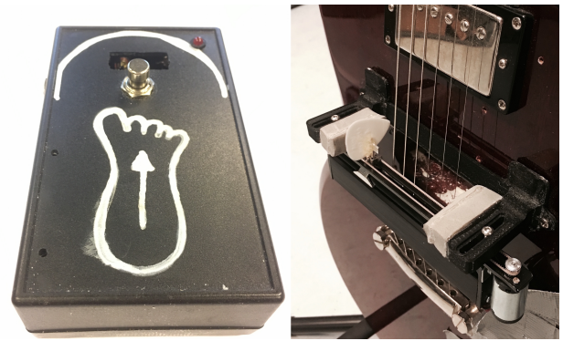
Figure 1: The pedal with the momentary button and built-in datalogger (left) and the electrical guitar with the motorised pick (right).
