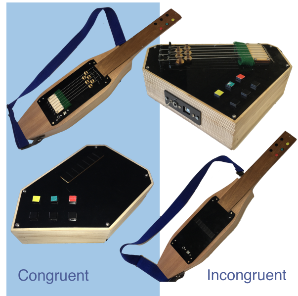
Figure 1: Four ‘guitar-like’ instruments. Clockwise from top left: Strings-Guitar (SG), Strings-Tabletop (ST), Touch-Guitar (TG) and Touch-Tabletop (TT). Congruent and Incongruent pairs are shown.
