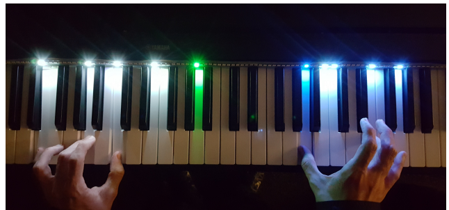
Figure 1: The Lumanote LED interface under dim lighting conditions.
