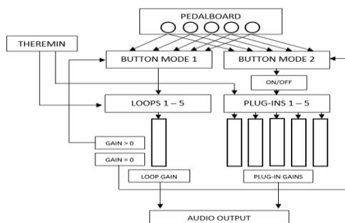
Figure 2. Signal Flow Diagram of Max/MSP Patch
