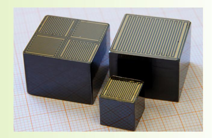
• Mean FWHM at 662 keV of installed detectors during evaluation for XDEM 2.4 % compared to 2.8 % for demonstrator phase, corresponding to about 1.3 % FWHM at  $Q_{\beta\beta}$  of <sup>116</sup>Cd
