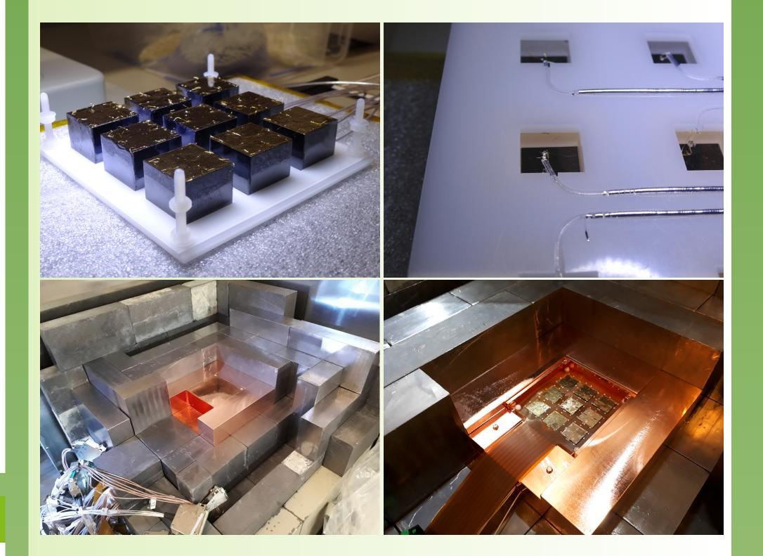
• Successful installation of detectors, working electrical contact for all channels, calibration with <sup>22</sup>Na and <sup>228</sup>Th
