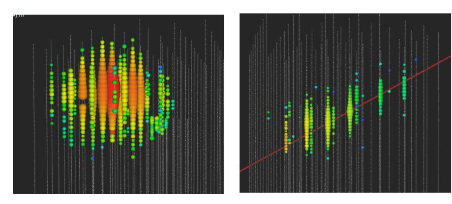
High energy event displays: ~ I PeV cascadetype (left) and  $\sim$  340 TeV muon-type (right)
