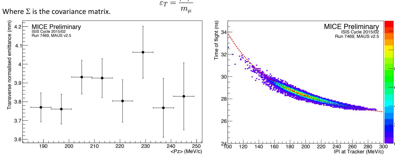
Figure 6: First direct measurement of emittance using the most upstream scintillating fibre tracker station [9].
