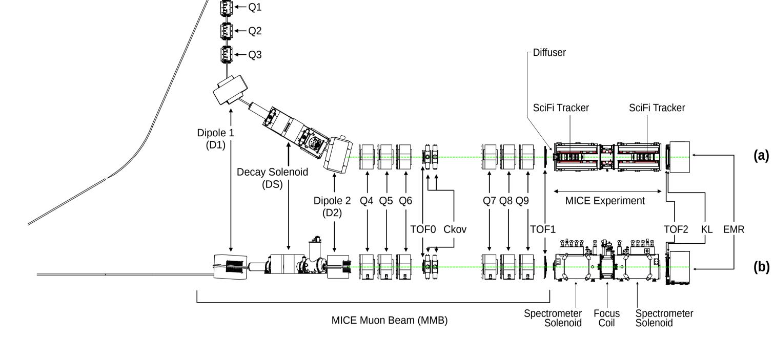
Figure 1: Schematic of the MICE beamline and MICE experiment [4]. (a) and (b) are the top and side views, respectively.
