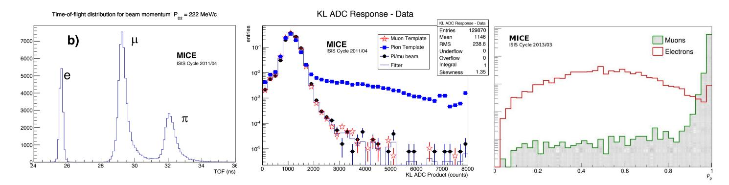
Figure 3: The measured electron, muon, Figure 4: Histogram of the KLOE-Light and pion time-of- flight distributions detector ADC count [5]. between the TOF0 and TOF1 detectors [5].
