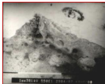
Fig. 5. Micrography using the MEB of the glaze/terra cotta interface zone of KBHEC08
