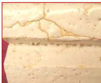
Fig. 1. Defect of withdrawal of the stalactite enamel KBHEC01
