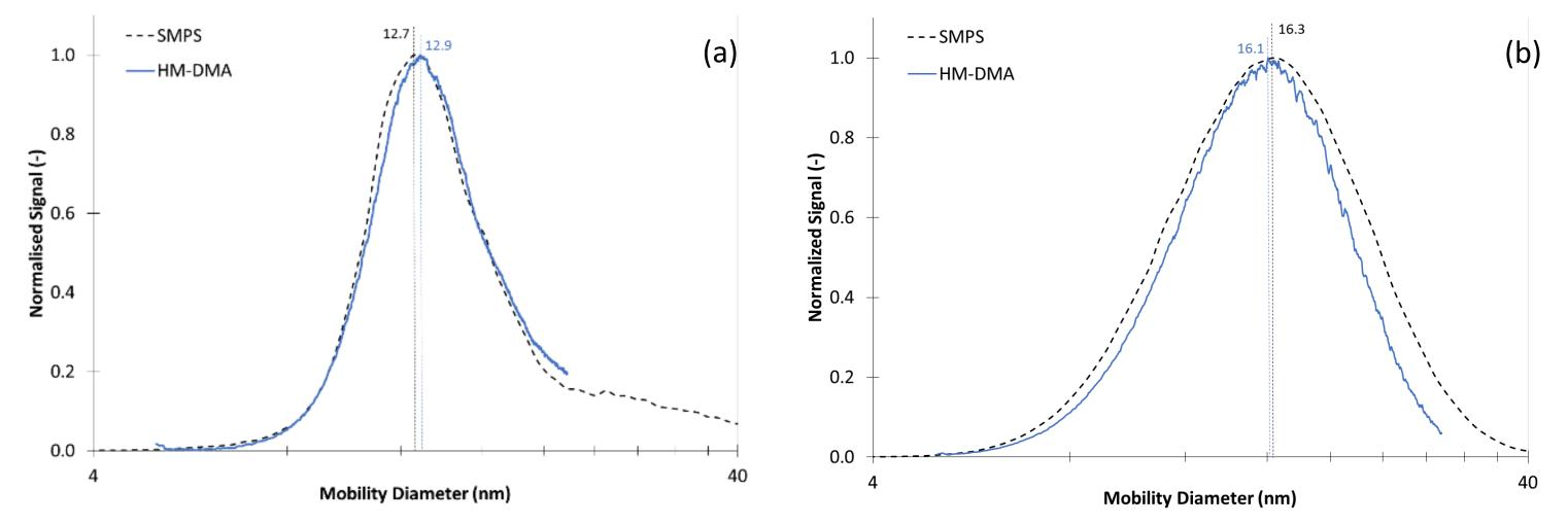
**Figure 2.** Normalized particle size distribution of (a) NaCl particles, and (b) CAST-generated soot particles, measured with *Advanced H-M DMA* at the hot temperature mode and compared with an SMPS (NanoDMA 3085, CPC 3776).
