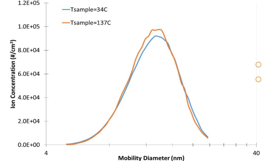
Identical d<sub>m</sub>=13.2 nm & σ<sub>g</sub>=1.3
