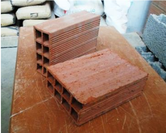
Fig 2. Clay bricks used.
