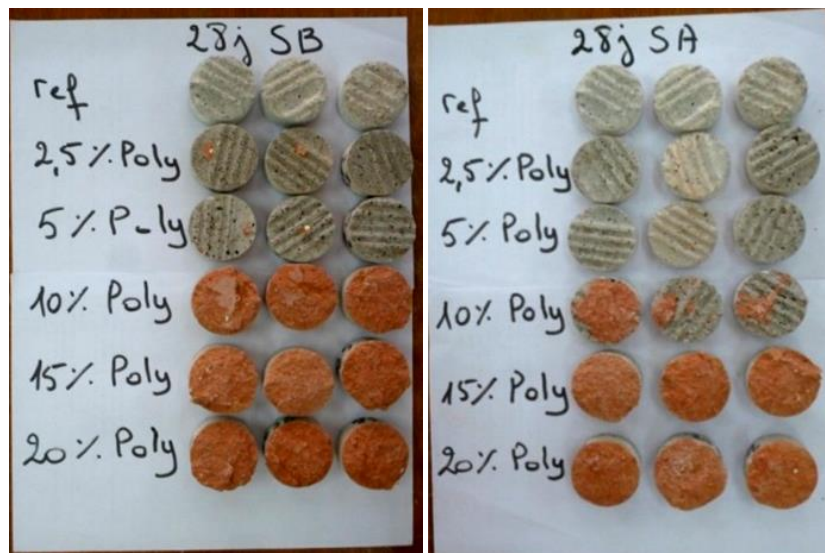
Fig 15. Failure mode of the samples clay bricks – mortars.
