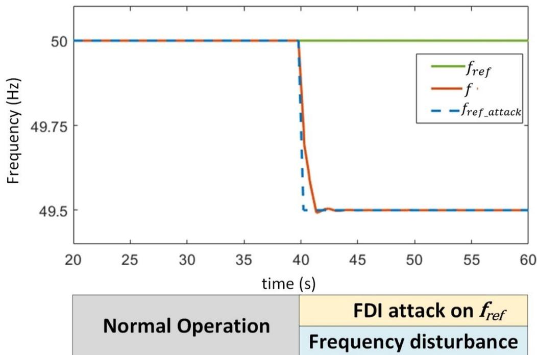
Figure 3: Microgrid operation during islanding mode, with an MITM-FDI attack on frequency reference signal  $f_{ref}$  between higher-level controller and microgrid local controller.
