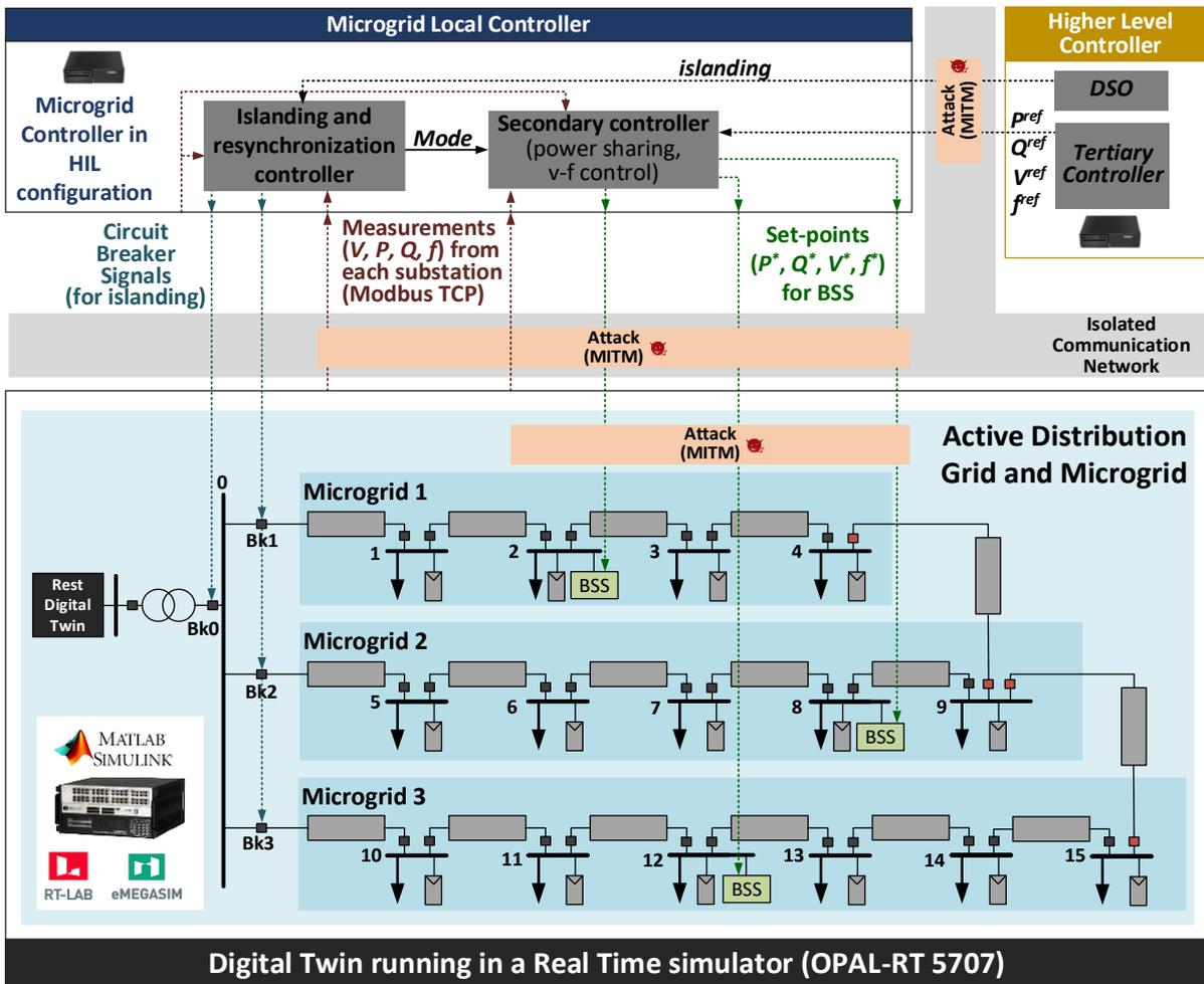
Figure 1 Testbed setup for investigating cyber-attack in active distribution grid and microgrid operation.
