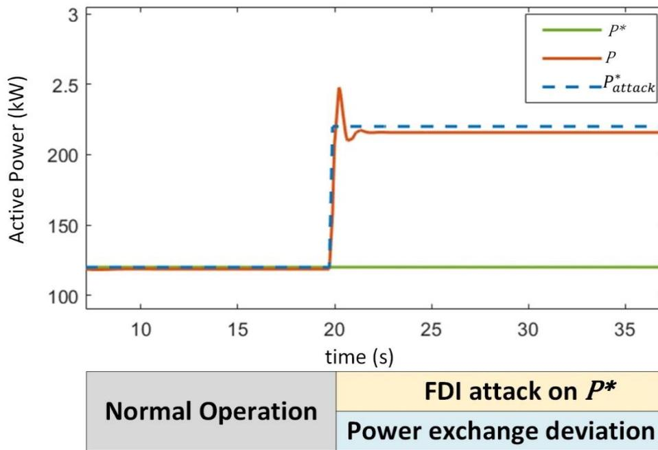
Figure 2: Active distribution grid operation during grid-connected mode, with an MITM-FDI attack on active power set-point  $P^*$  between microgrid local controller and BSS.
