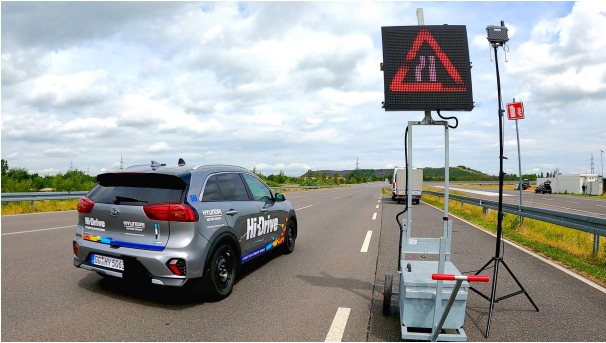
Fig. 7. CAV Prototype and RSU used for real-world validation
