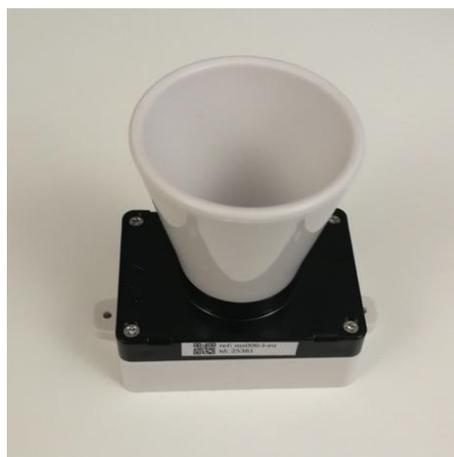
*Fig. 13 – LoRaWAN ultrasound presence sensor*
