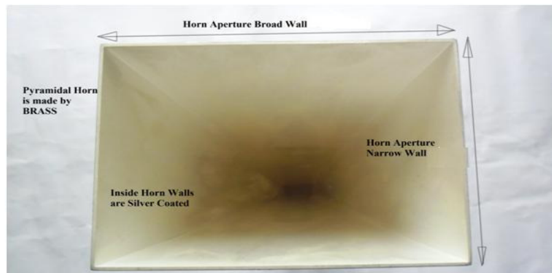
Figure 14. Designed Aperture of Pyramidal Horn dimensions
