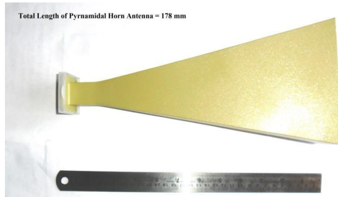
Figure 13. Fabricated Pyramidal Horn Antenna
