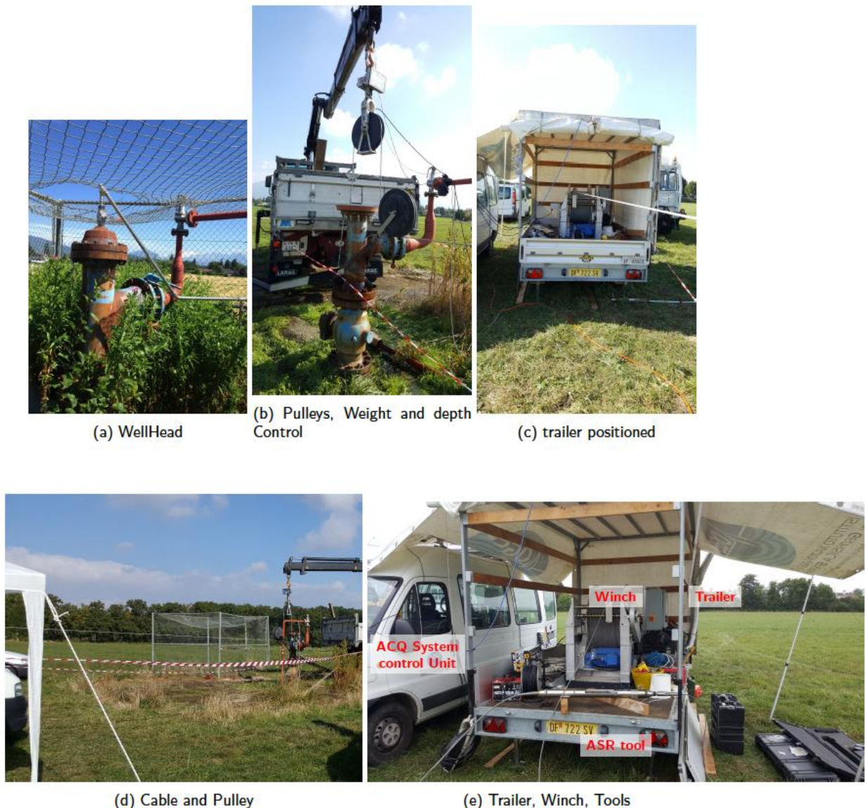
Fig. 7 – Move in and installation operation for the second phase
