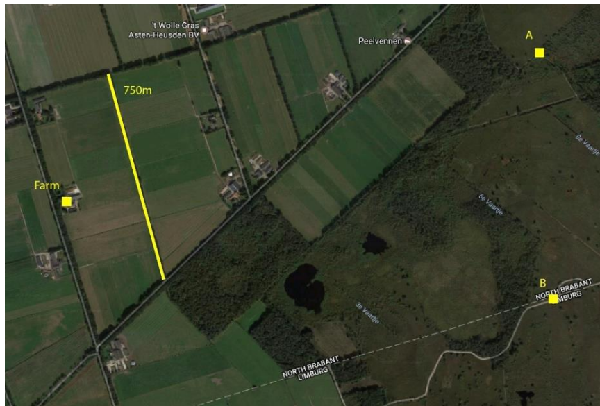
Figure 158 - Satellite image of the survey area, with the 750 m receiver line coloured yellow. The equipment was controlled from the indicated farm slightly west of the line. Points A and B represent the locations of two borehole surveys. From Google Maps (2017).
