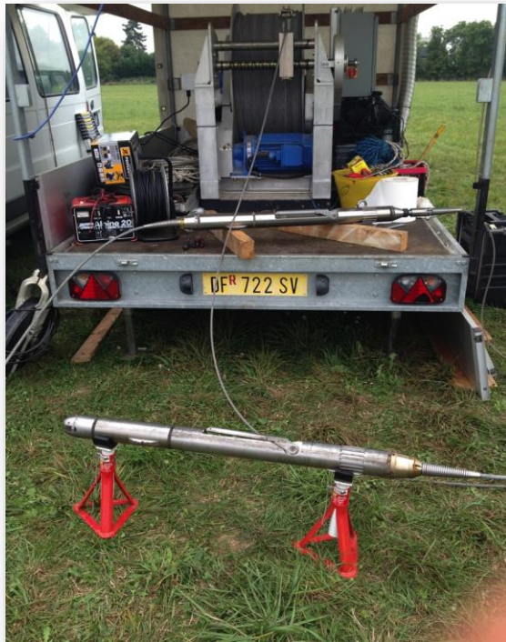
Figure 110 : Two levels tool strings used to acquire the survey
