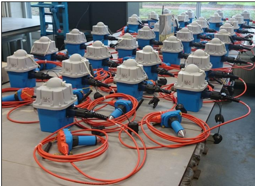
Figure 165 - Seismic stations in the workshop at TNO, Utrecht. The DSU-3 units are the smaller components with the metal point and orange top. The RAU-D units have a grey top with a small dome.
