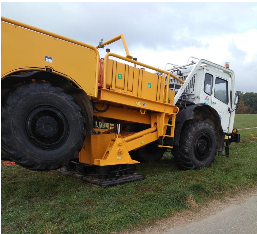
Figure 111 : Prakla vibroseis used as energy source for the VSP survey
