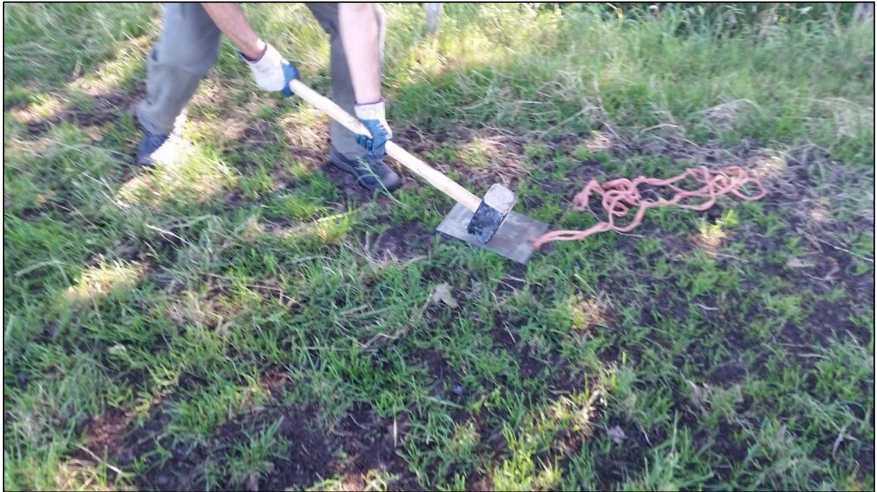
Figure 169 - Active seismic acquisition using a hammer and a metal plate.
