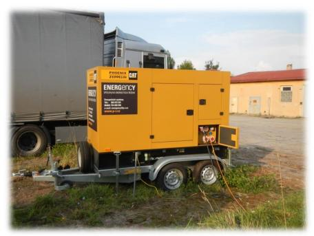
Figure 16 : 50 kVA power generator.
