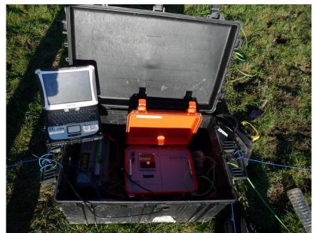
Figure 19 : Recording device (ADU07 in orange)
