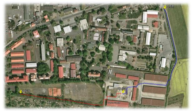
Figure 12 - Location of current injection poles. U and V are surface injection points and W is a 1.8 km long metallic casing borehole (Google Earth image).
