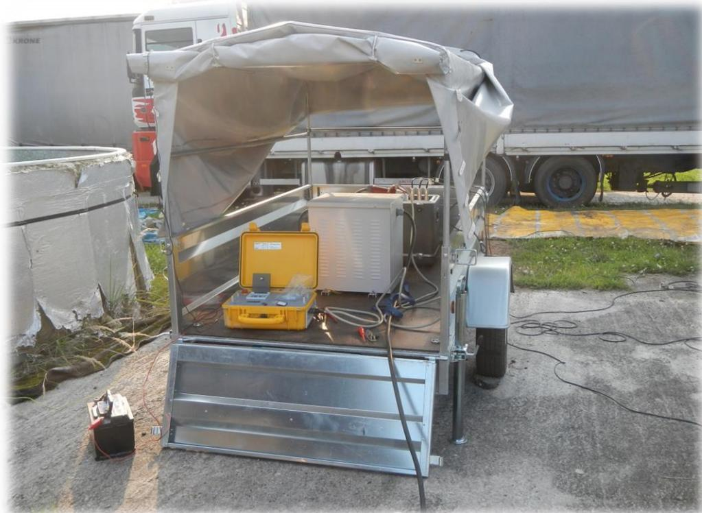
**Figure 15 : Transmitter TXM22 with TXB07 controller.**
