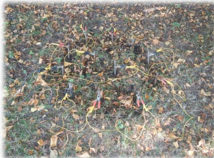
**Figure 13 : Surface electrode (E1).**
