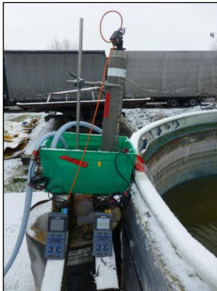
Figure 4 - Close view of the Idronaut probe used for continuous physico-chemical monitoring during pumping; portable multi-meters for spot data acquisitions are also visible (bottom part of the image).
