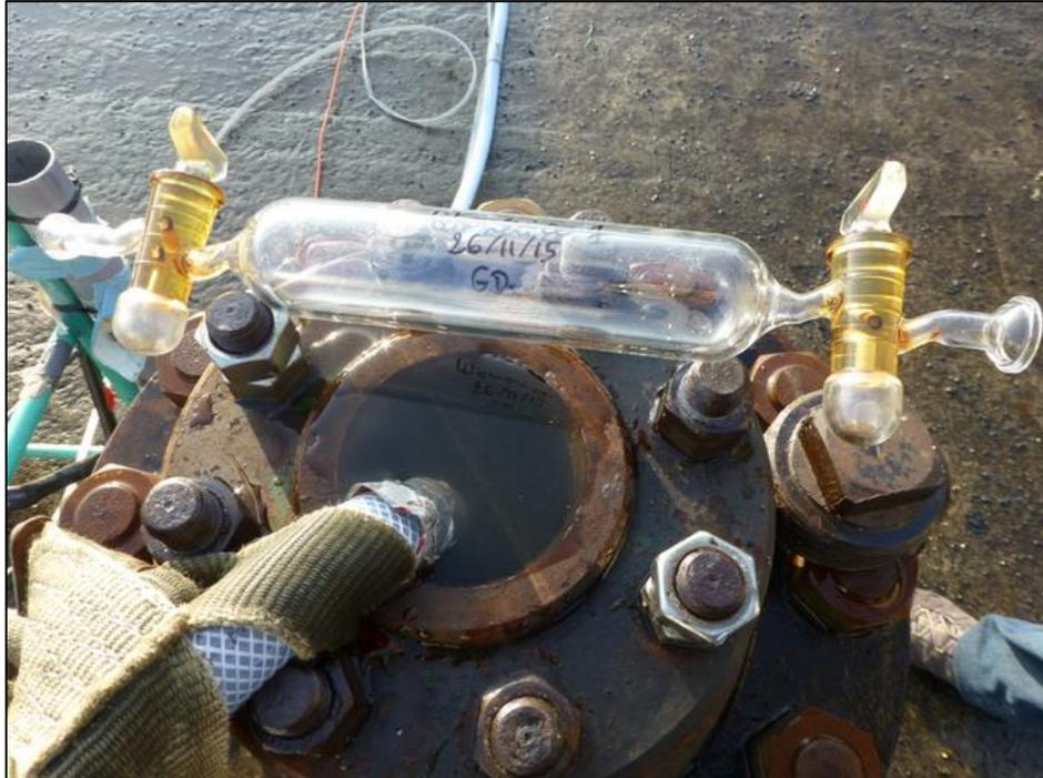
Figure 11 - Glass bulb under vacuum prior its use for collection of dissolved gases.
