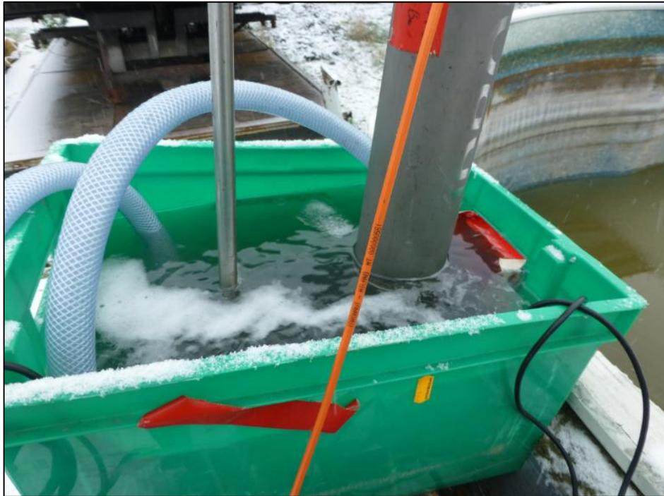
Figure 10 - Degassing of the water during a pumping session.
