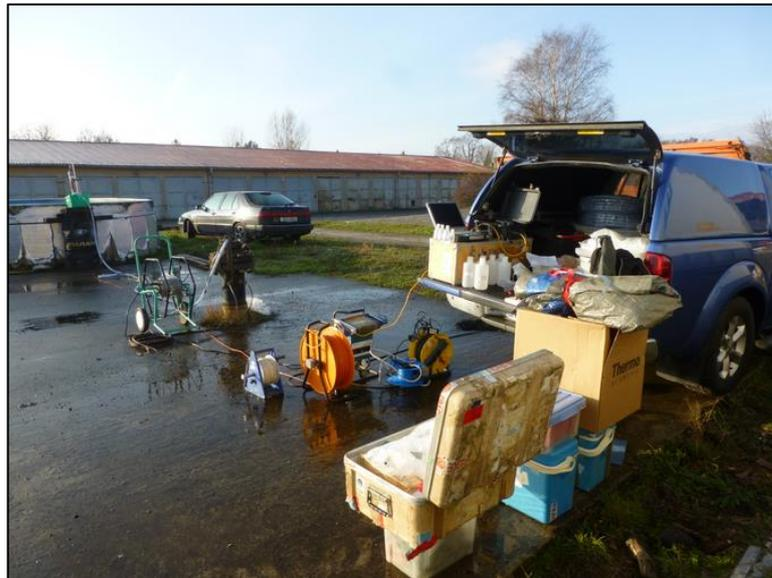
Figure 2 - Overview of the field operations; left: multi-parameter probe and pool for discharge of pumped water; middle: borehole and pumping system; right: material for physico-chemical monitoring and material for sampling water.
