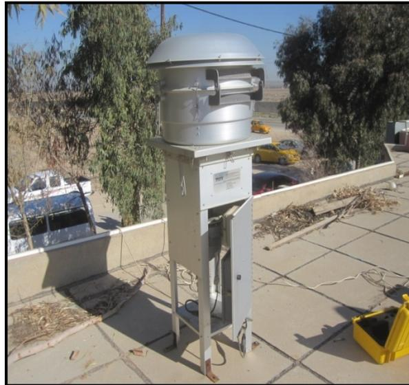
**Figure 4:** Hi-volume air sampler
