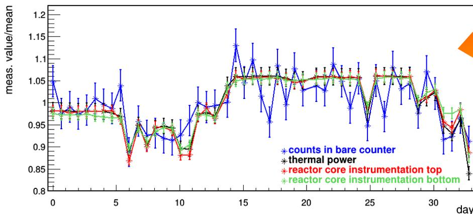
1. Neutron field **highly thermalized** (>80%), correlated with thermal power
