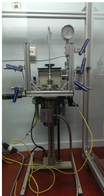
Figure 5. Pictures of experimental setup for thermal stability experiments at supercritical water conditions.
