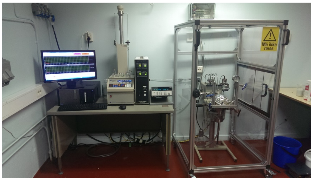
Figure 6. Picture of experimental setup for thermal stability experiments at supercritical water conditions.
