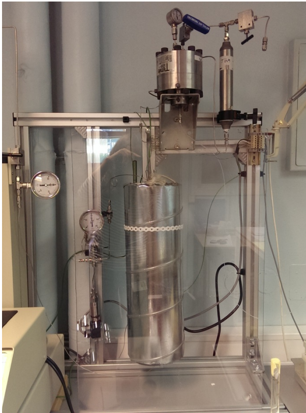
Figure 9. Picture of the high temperature oven and the back pressure regulator of the dynamic setup.
