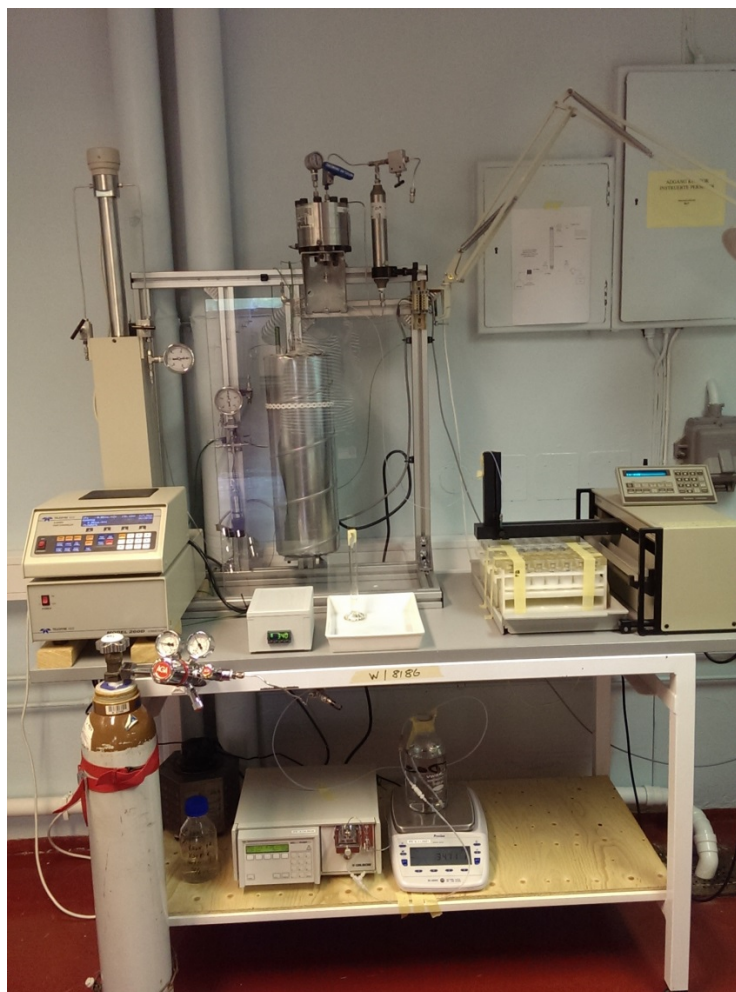
Figure 8. Experimental setup for dynamic experiments with selected tracer candidates. The system consists of a piston cylinder containing the tracer mixture, a pump, a packed column inside a heating unit, a coil for cooling water prior to sampling, a backpressure regulator and a sampling unit.
