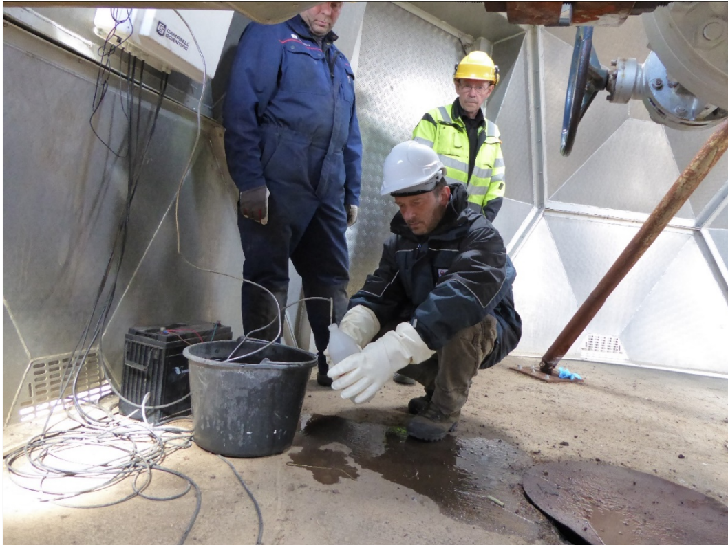
Figure 1. Collecting samples from well KJ-39, the injection well – before mixing the tracers.
