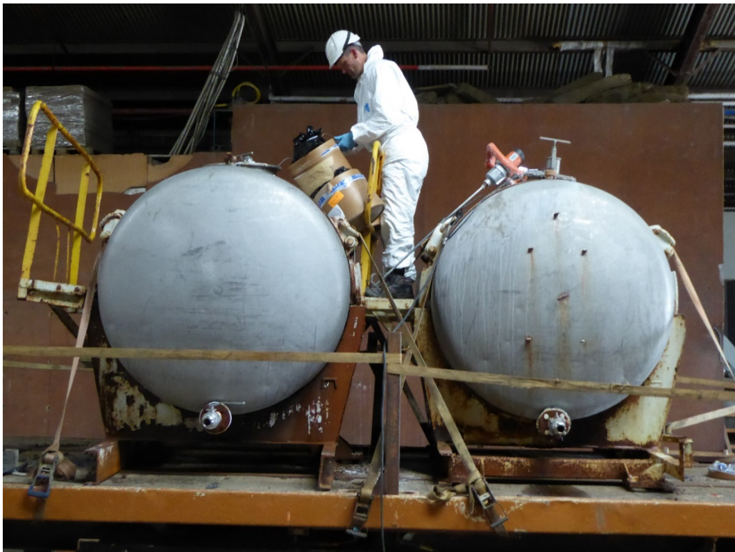
Figure 3. Preparing to add the tracers gently into the tanks.
