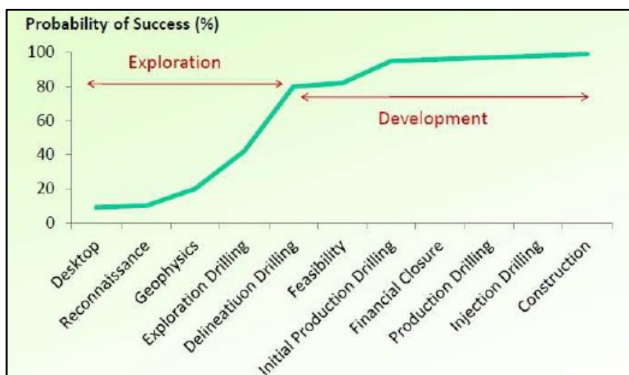
Figure 1: Variation of risks at different phase of a geothermal project (Source GEA 2008)
