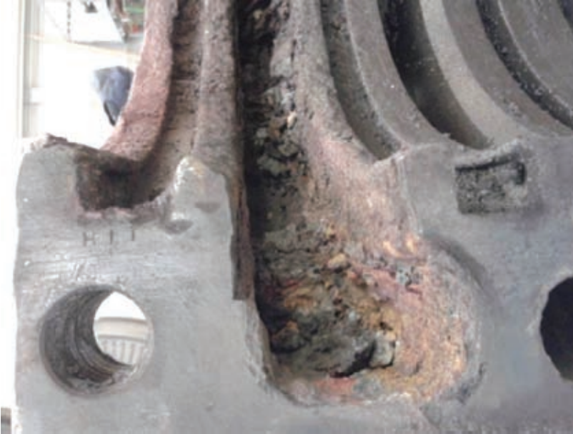
Figure 4. Scaling and corrosion in turbine casing
