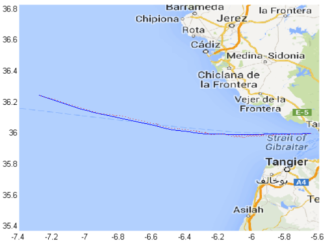
Figure 7. Tracks of cluster centroids. The blue line indicates the cluster path of the ground truth convoy of ships; the dashed red line is the cluster path after processing the combined ship traffic. The two clusters merged or stayed very close to each other.
