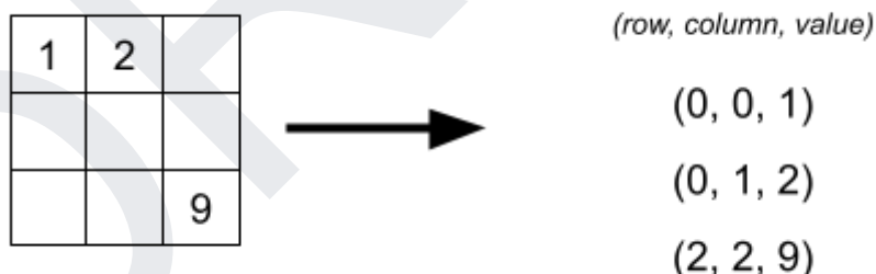
Figure 14: An example sparse matrix converted into an equivalent set of tuples.
