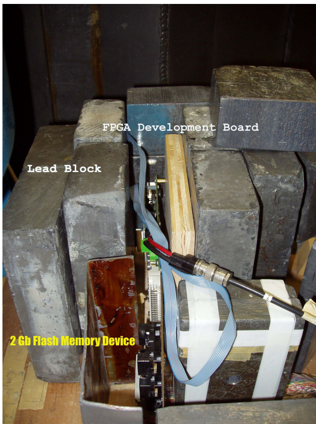
Fig. 4: TID in-situ test setup at the JPL Cobalt-60 facility
